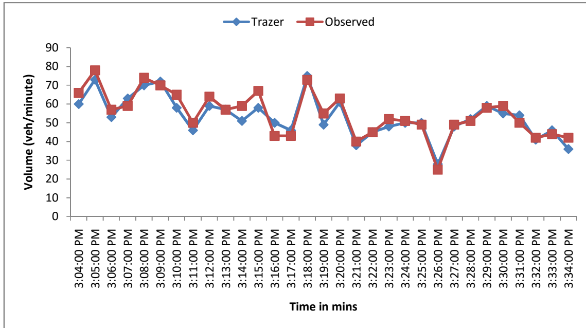
Figure 86: Comparison of actual volume and Trazer volume during off-peak condition
