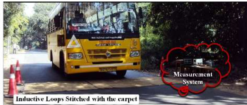
Figure 156: Experimental setup used for conducting field studies with six inductive loops stitched to a carpet.
