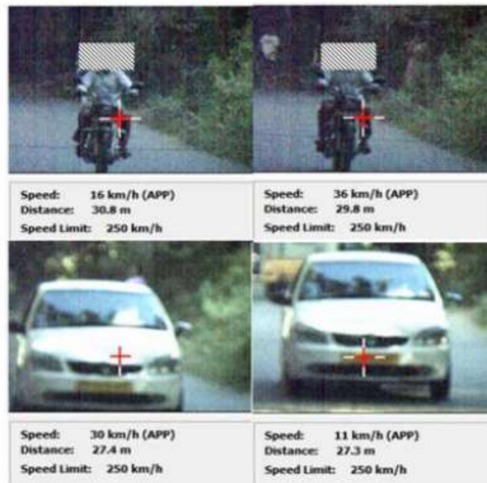
Figure 132: Speed given by the laser gun during the test. This is used as the reference measurement
