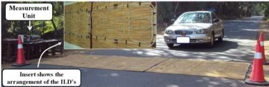
Figure 148: Shows the snap-shot of the detector system covering the entire road width. The Inductive Loop Detectors (ILD) stitched to a carpet is shown in inset picture.
