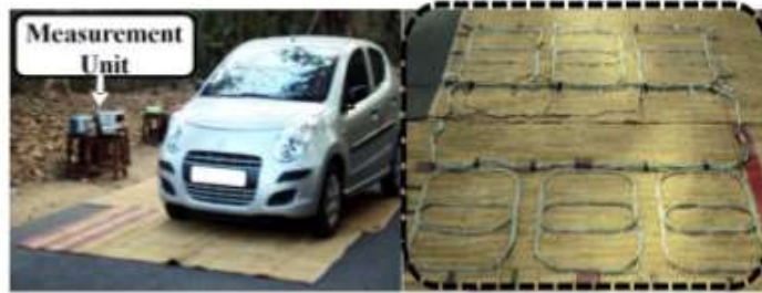
Figure 152: Photographs of the experimental set-up (left) and the new configuration of the loop system stitched to the carpet (right).
