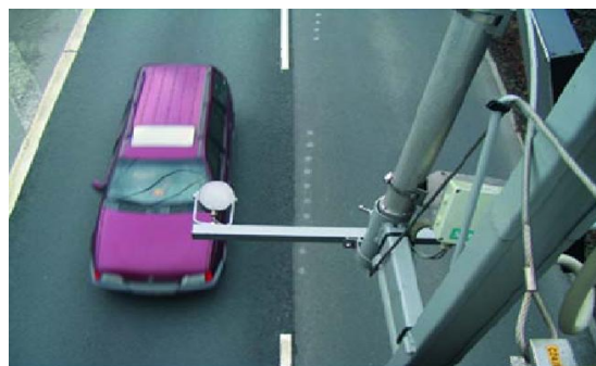
Figure 11: Passive IR Detector [16]
