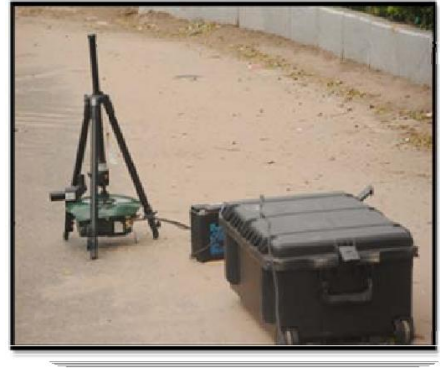
Figure 43: The portable TIRTL used in this study
